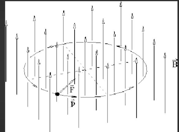
*Motion of an electron (negative charge) in a uniform magnetic field.*
